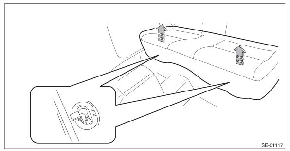
(2) Remove the hook (A) by pushing it back while lifting the front side of the seat cushion, and remove the seat cushion.
