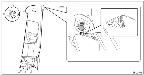
(4) Pull out the seat belt and remove the center pillar trim UPR.
