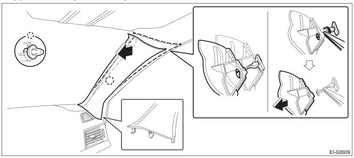
2) Release the claws, and then remove the side sill cover-front INN.
