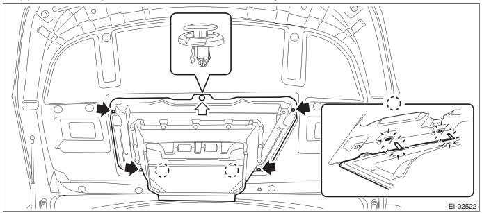
3) Release the clips to remove the front hood insulator.
