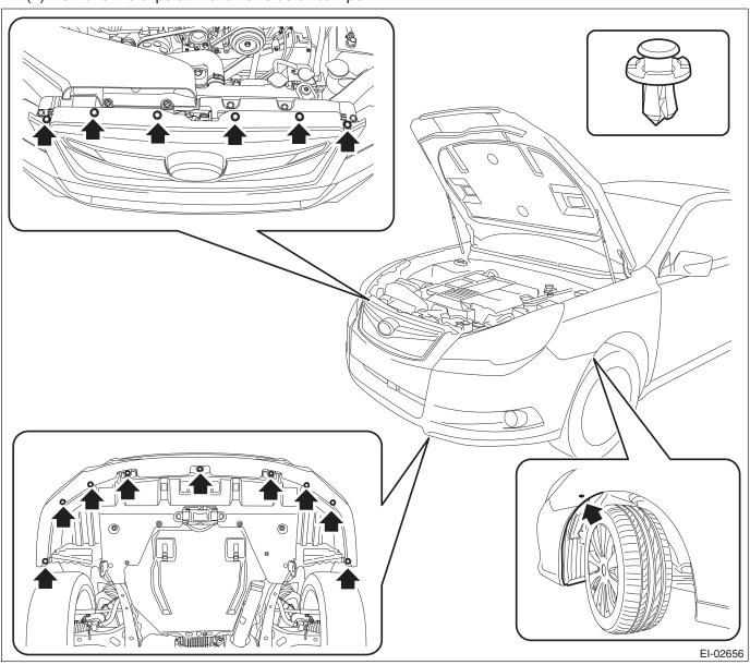
(5) Detach the flange section on the bumper face side from the bracket side front UPR.
