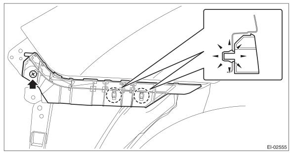
6) Remove the bolts and pins, and remove the front fog light assembly.
