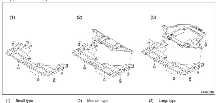
(2) Remove the clip, and remove the bracket center LWR-front.
