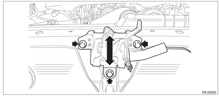
Tightening torque: 33 N·m (3.36 kgf-m, 24.3 ft-lb) 3) Rotate the hood buffer to adjust lateral height.
