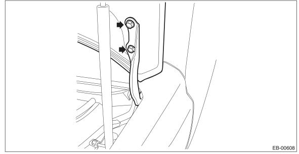
(2) Adjust the horizontal panel gap of the front hood and tighten the hinge attaching bolts.
