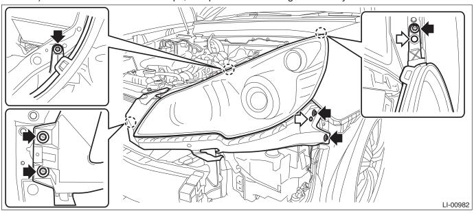
b) Disconnect the connector and remove the headlight assembly.
