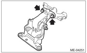
3) Install the turbocharger upper stay to the engine mounting bracket.
