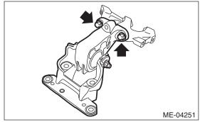
3) Remove the front cushion rubber from the front mounting bracket.
