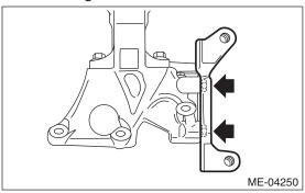
2) Remove the front cushion rubber from the engine mounting bracket.
