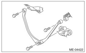
12) Remove the bolt and nut which secure engine mounting to the cradle.
