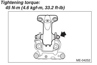
2) Install the front cushion rubber to the engine mounting bracket.
