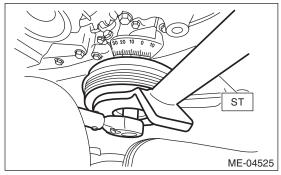
(2) Draw reference lines (A) and (B) using a marker to set the socket to the crank pulley bolt as shown in the figure.
