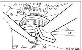
5) Install the V-belts. <Ref. to ME(H4DOTC)-42, INSTALLATION, V-belt.>
