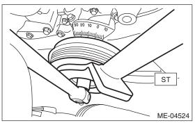
3) Remove the crank pulley.
