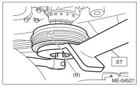
(4) Use the ST to lock the crank pulley, and tighten the crank pulley bolt to the angle where reference line (A) and end line (C) are aligned.
