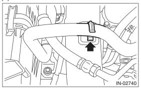
(6) Disconnect the connector (A) from power steering pump, and remove the power steering pump together with the power steering pump bracket from engine and rod stopper.
