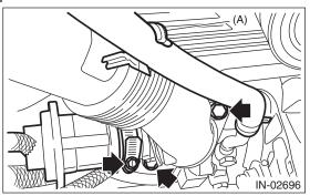
(11) Remove the intake duct from intake manifold.
