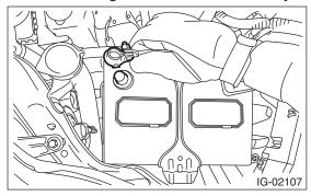
3) When removing the timing belt cover RH(1) Remove the air intake duct. <Ref. to IN(H4DOTC)-12, REMOVAL, Air Intake Duct.>(2) Loosen the clamp which holds the intake duct to intercooler.
