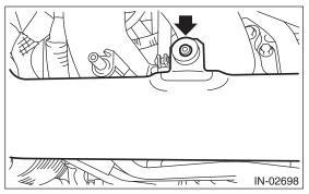
(12) Disconnect the vacuum hose from blow-by pipe, and remove the bolt securing the blow-by pipe from the intake manifold protector RH.
