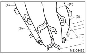
4) Remove the clip which holds the engine harness to the hose clip stay assembly.
