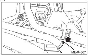
(14) Remove the vacuum hose (A), vacuum hose (B), vacuum hose (C) and vacuum hose (D) from the clip (E).
