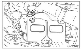
3) Remove the oil pressure switch. <Ref. to LU(H4SO)-23, REMOVAL, Oil Pressure Switch.> 4) Attach the oil pressure gauge to the cylinder block.
