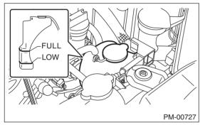
3) Remove the radiator cap and make sure that the radiator is filled with engine coolant up to the filler neck position.
