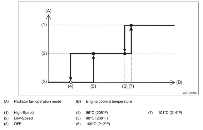
• Radiator fan operation mode related to A/C compressor load
