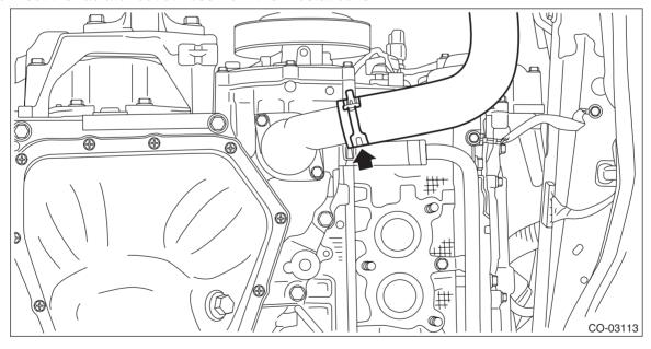
7) Remove the thermostat cover, and then remove the gasket and thermostat.
