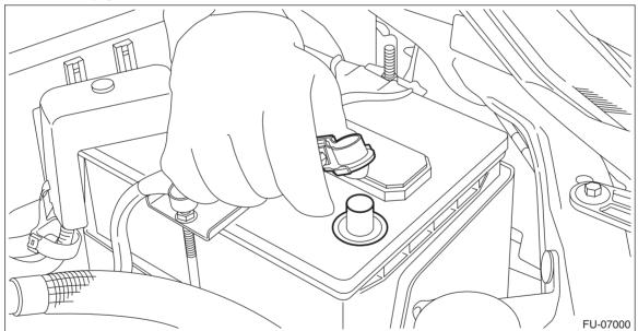
8) Fill engine coolant. <Ref. to CO(H4DO)-15, FILLING OF ENGINE COOLANT, REPLACEMENT, Engine Coolant.>
