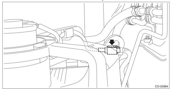
4) Remove the CVTF radiator hose from the clip of the radiator main fan shroud. (CVT model)
