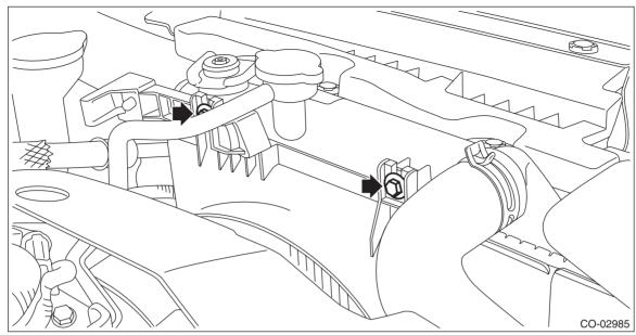
6) Remove the radiator main fan and fan motor from vehicle.
