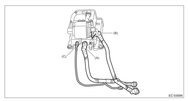
3) Install the canister to the vehicle, and connect the connector (A) to the canister.
