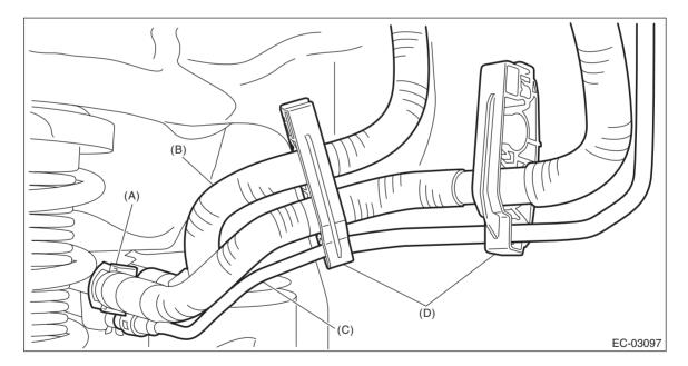
6) Disconnect the connector (A) from the canister and remove the canister from the vehicle.
