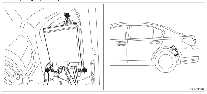
4) Attach all tubes to tube clamp (D), and connect the quick connectors of the vent tube (A), canister drain tube (B) and charge tube (C).
