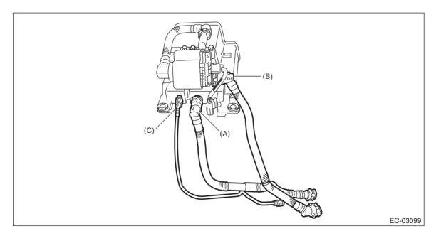
8) Disconnect the connector (A) from the leak check valve assembly, and remove the connector assembly from the canister clip.
