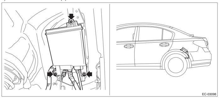
7) Disconnect the vent tube (A), canister drain tube (B) and charge tube (C) from the canister.
