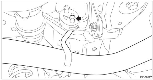
3) Install the rear exhaust pipe to the muffler.
