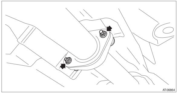
3) Remove the muffler from rear exhaust pipe.
