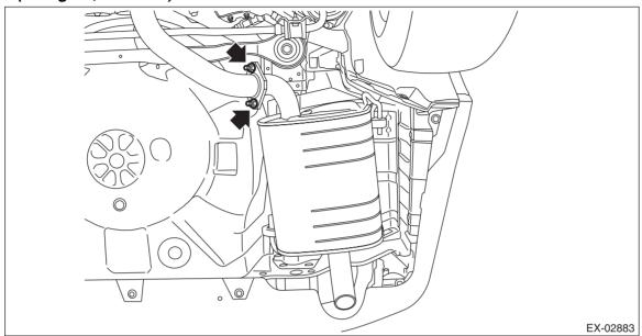
4) Install the center exhaust pipe to rear exhaust pipe.
