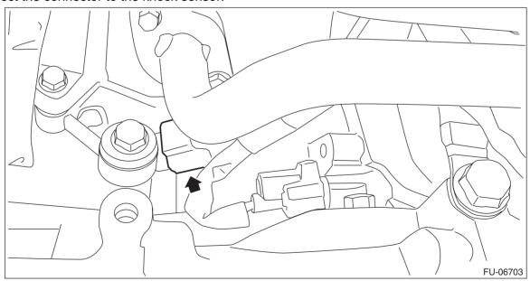
3) Install the air intake boot. <Ref. to IN(H4DO)-13, INSTALLATION, Air Intake Boot.>
