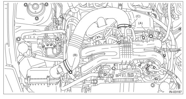
5) Remove the air intake boot from the throttle body, and move it to the left side wheel apron.
