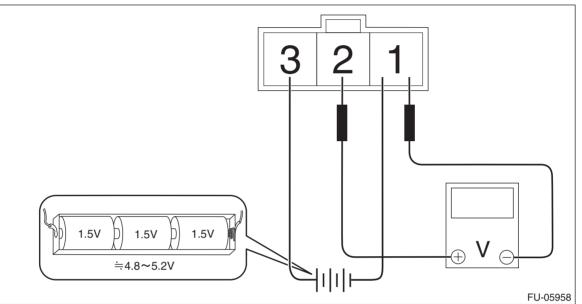
3) Check the voltage at a normal atmospheric pressure.
