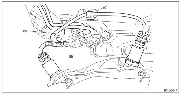
(A) Front oxygen (A/F) sensor con- (B) Rear oxygen sensor connector (C) Clip nector
