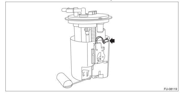
4) Press two claws (A) of the fuel level sensor, and slide the fuel level sensor in the direction of the arrow to remove the fuel level sensor.
