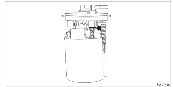
3) Remove the harness from the claw of fuel chamber assembly.
