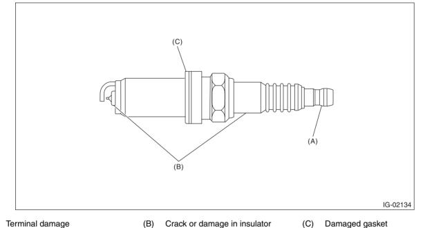
2) Check the spark plug electrode and condition of the insulator. If abnormal, check and repair the cause and replace the spark plug.
