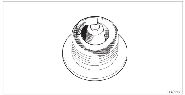
3) Using a nylon brush, etc., clean and remove the carbon or oxide deposits from the spark plug. If deposits are too stubborn, replace the spark plugs. After cleaning the spark plugs, check the spark plug gap "L" using a gap gauge. If it is not within the standard, replace the spark plug.
