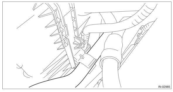
4) Disconnect the connector (A) from the mass air flow and intake air temperature sensor, and remove the clip (B).
