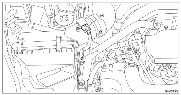
5) Loosen the clamp (A) which connects the air cleaner case (rear) and air intake boot, and then remove the clip (B) from the air cleaner case (front).
