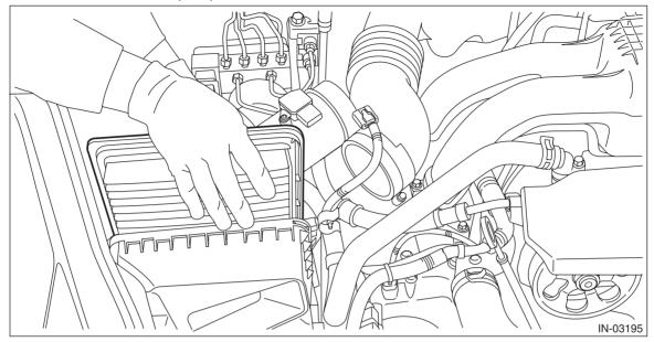
7) Remove the bolt (A) and nut (B) which secure the air cleaner case (front) to the body.
