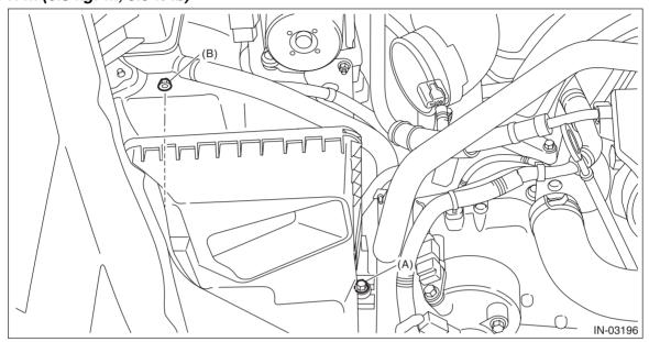
2) Install the air cleaner case (rear) and air cleaner element.
