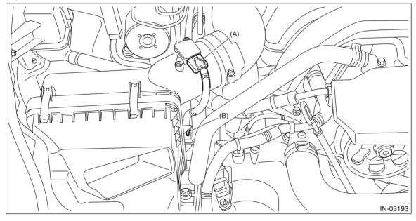
5) Connect the power steering oil pressure hose (suction hose) to the clip on the side of air cleaner case (rear).
