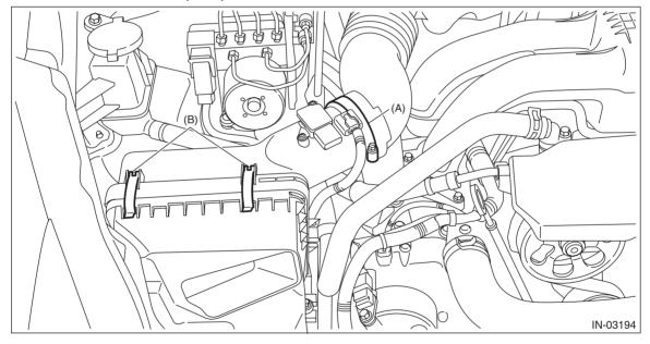
6) Remove the air cleaner case (rear) and air cleaner element.
