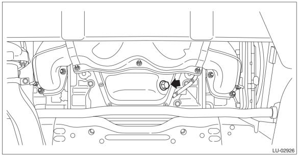
4) After draining the engine oil, tighten the engine oil drain plug.
