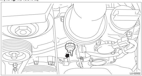
3) Connect the terminal to the oil pressure switch.
