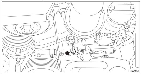
3) Remove the oil pressure switch.
