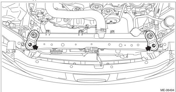
9) Slide the radiator to the right and left, and remove the front mounting bracket.
