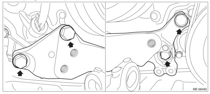
6) Install the front cushion rubber to the front mounting bracket and engine mounting bracket.
