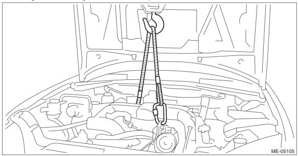
5) Remove the front cushion rubber from the front mounting bracket and engine mounting bracket.
