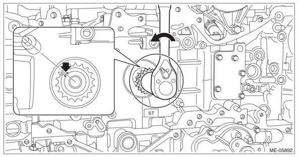
5) Align the alignment mark of exhaust cam sprocket LH to the position shown in the figure.
