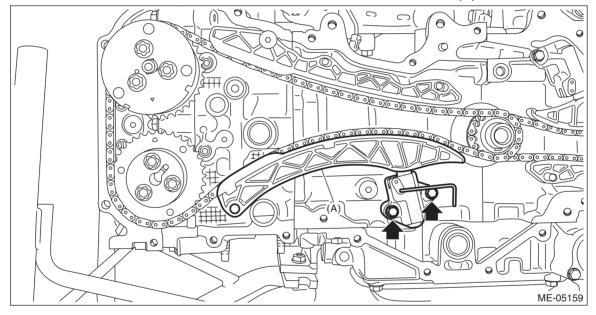
5) Remove the chain guide RH, and remove the timing chain RH (A).
