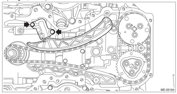
9) Pull out the stopper pin from the chain tensioner LH.
