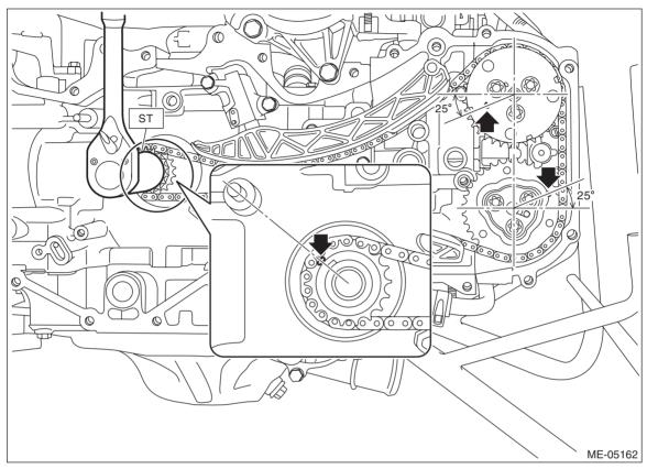
3) Push down the chain lever tensioner LH, and with a 2.5 mm (0.98 in) dia. stopper pin or a 2.5 mm (0.98 in) dia. hex wrench inserted into the stopper pin hole in the chain tensioner LH, secure the plunger (A).
