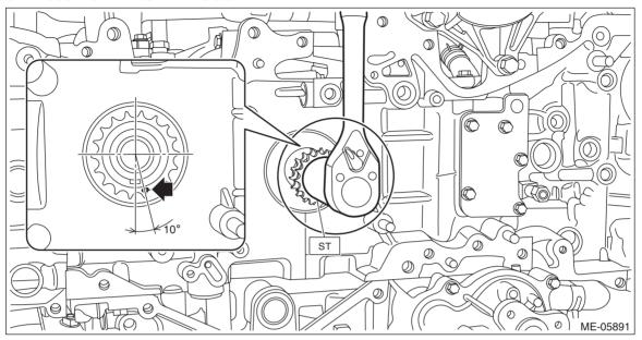
3) Using ST and by turning the intake cam sprocket LH, align the alignment marks to the positions as shown in the figure.
