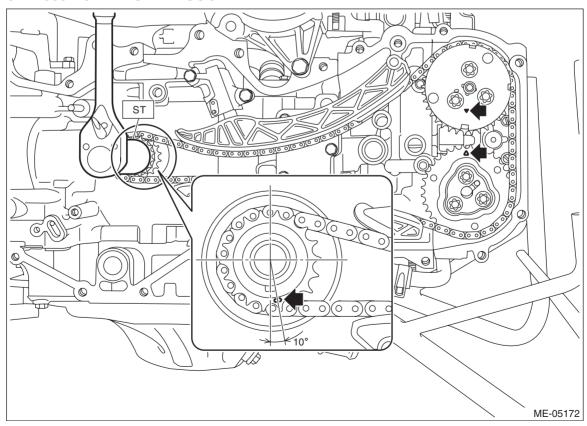
12) Install the timing chain RH. <Ref. to ME(H4DO)-126, TIMING CHAIN RH, INSTALLATION, Timing Chain Assembly.>
