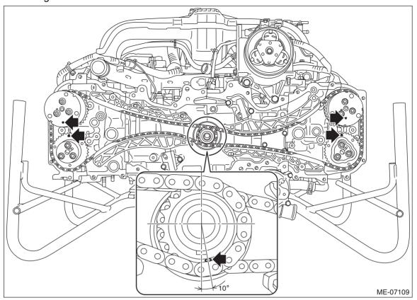
9) Using the ST, turn the crankshaft clockwise, and make sure that there are no abnormal conditions.
