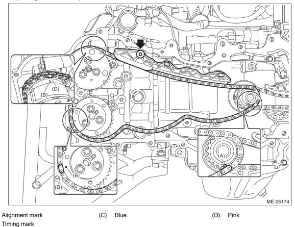
6) Install the chain tensioner lever RH (A) and chain tensioner RH.
