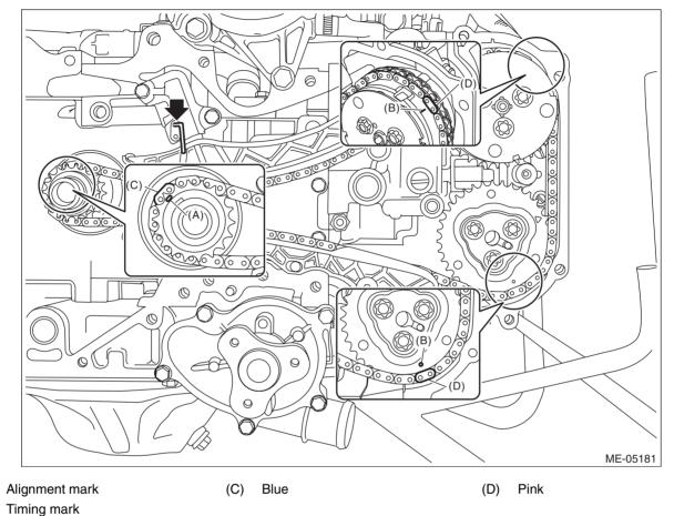
10) Using the ST, turn the crankshaft clockwise, and make sure that there are no abnormal conditions.
