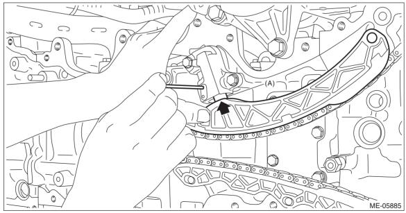
4) Remove the chain tensioner LH, and remove the chain tensioner lever LH (A).
