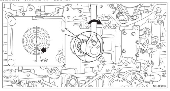
8) Using ST and by turning the intake cam sprocket LH approximately 180°, align the alignment marks of intake cam sprocket LH to the positions (zero-lift position) as shown in the figure.
