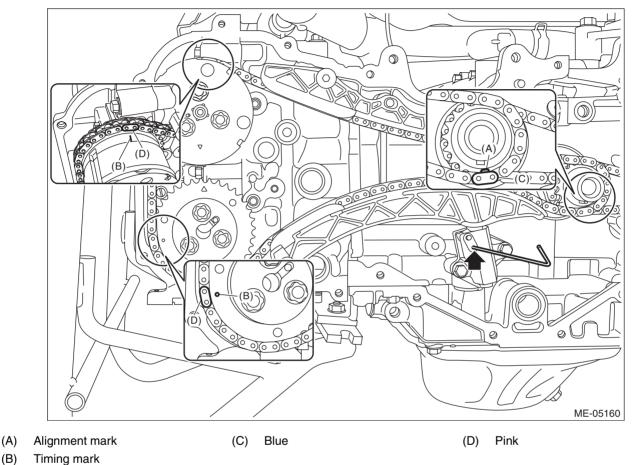
8) Make sure that the alignment marks of the cam sprocket and crank sprocket are aligned to the positions as shown in the figure.
