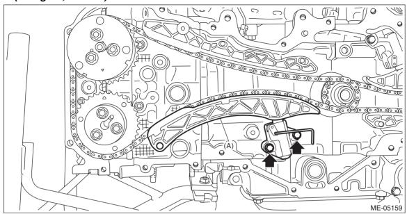
7) Pull out the stopper pin from the chain tensioner RH.
