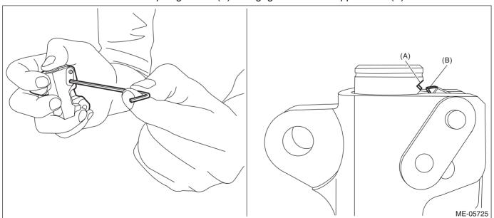
2) Check that the crank sprocket is located at the position sown in the figure. If not aligned, using ST turn the crankshaft to align the crank sprocket alignment mark to the position shown in the figure.
