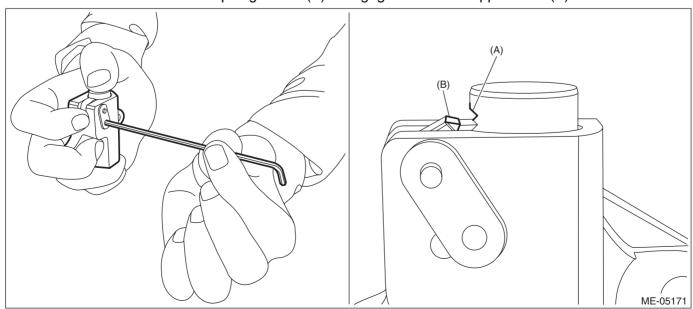
3) Make sure that the alignment marks of the crank sprocket, intake cam sprocket LH and exhaust cam sprocket LH are aligned to the positions as shown in the figure.
