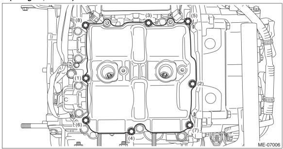
5) Install the intake manifold protector RH.
