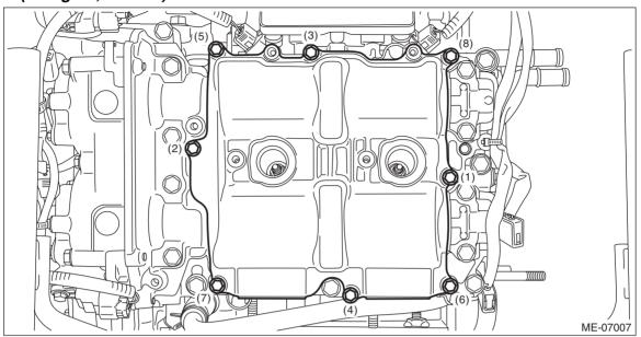
6) Install the intake manifold protector LH.
