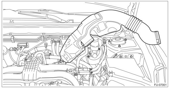
(4) Remove the front exhaust pipe. <Ref. to EX(H4DO)-5, REMOVAL, Front Exhaust Pipe.> 2) Remove the #1 ignition coil and the #3 ignition coil. <Ref. to IG(H4DO)-9, REMOVAL, Ignition Coil.>
