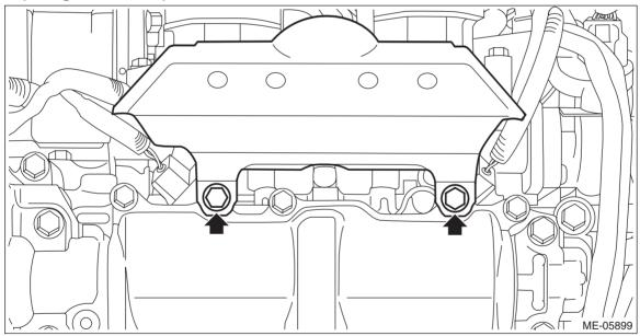
7) Install the #2 ignition coil and the #4 ignition coil. <Ref. to IG(H4DO)-9, INSTALLATION, Ignition Coil.>
