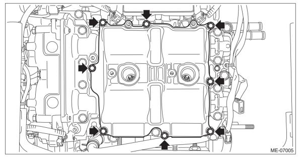
5) Remove the rocker cover gasket LH, #2 spark plug pipe gasket and #4 spark plug pipe gasket, and remove the liquid gasket.
