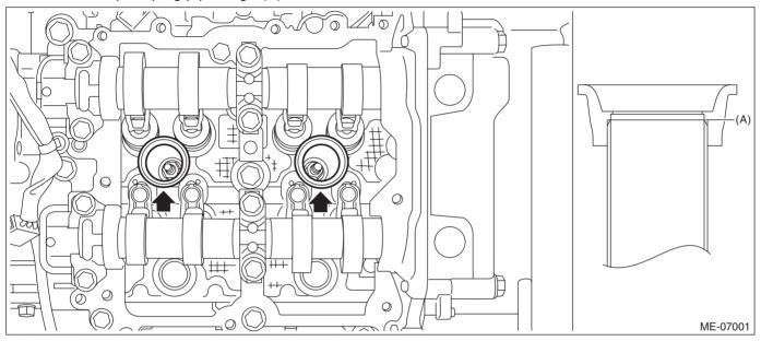
2) Install the rocker cover gasket RH to the rocker cover RH.
