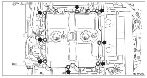
5) Remove the rocker cover gasket RH, #1 spark plug pipe gasket and #3 spark plug pipe gasket, and remove the liquid gasket.
