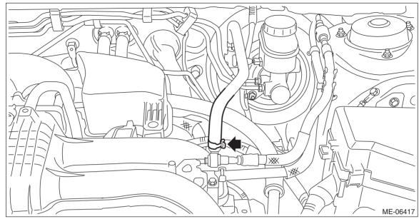
3) Connect the vacuum gauge to the intake manifold.
