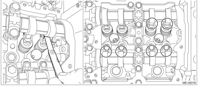
(4) Turn the crank pulley by 360°.
