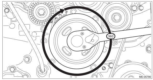
(5) Check the clearance of #4 cylinder intake.
