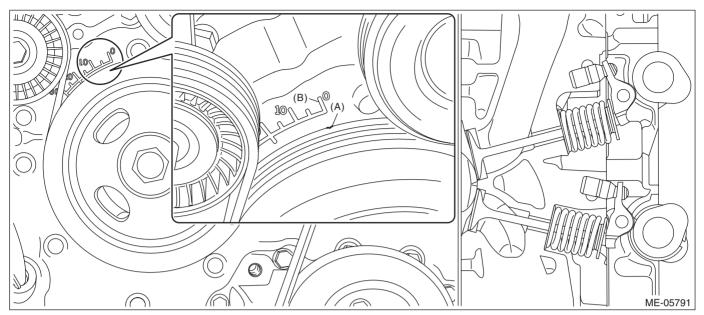
(3) Check the cam clearance for #2 cylinder intake, #2 cylinder exhaust and #4 cylinder exhaust.
