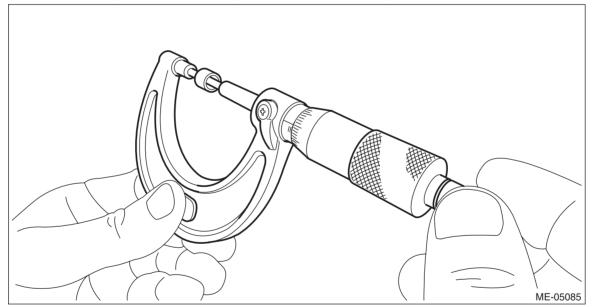
(4) Select a valve shim of suitable thickness using the measured cam clearance and valve shim thickness.
