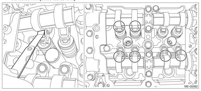
(4) Turn the crank pulley by 360°.
