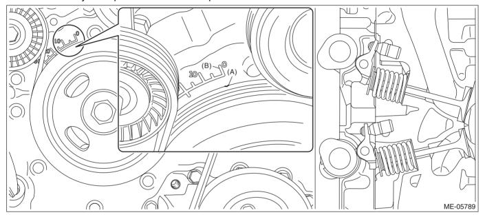
(3) Check the cam clearance for #1 cylinder intake, #1 cylinder exhaust and #3 cylinder exhaust.
