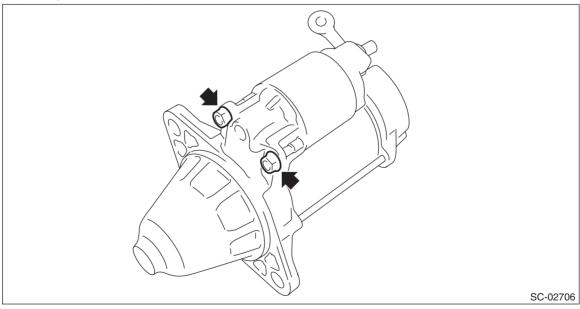
10) Install the harness to the terminal M (A) of the magnet switch assembly, and tighten the nut.
