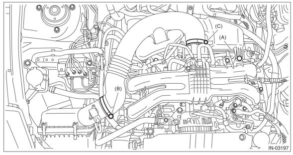
5) Remove the air intake boot from the throttle body, and move the air intake boot to the left side wheel apron.
