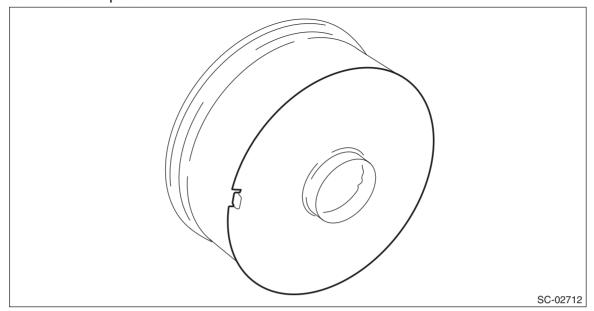
5) Assemble the overrunning clutch assembly to the yoke.
