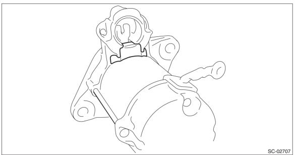
4) Remove the through bolts on both sides, and remove the starter housing.
