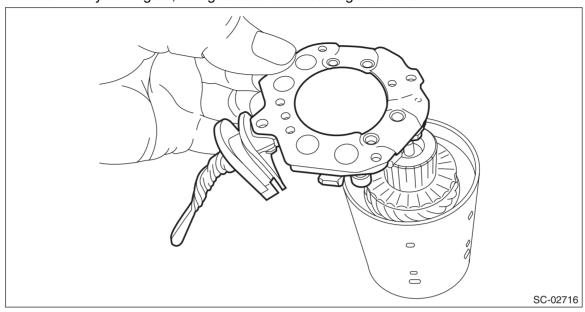
11) Remove the armature from the yoke.
