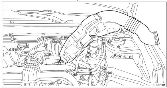
6) Disconnect the connector (B) and terminal (A) from starter.
