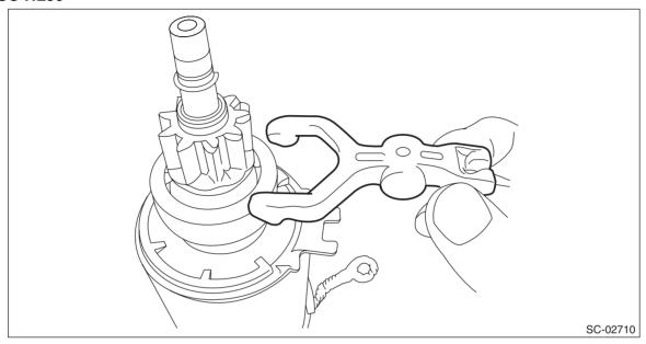
7) Install the starter housing, and tighten through bolts on both sides.
