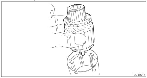
2) Install the brush holder assembly to the armature.
