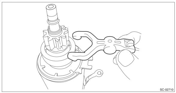
6) Remove the overrunning clutch assembly from the yoke.
