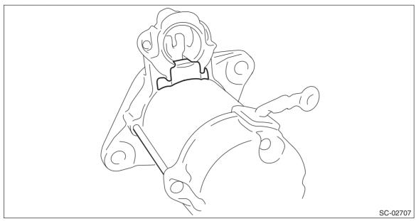
9) Install the magnet switch assembly to the starter housing, and tighten the nuts.
