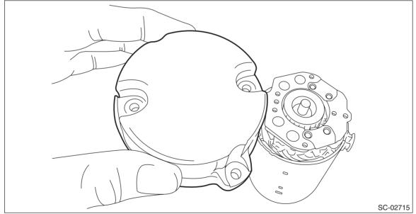
10) Remove the brush holder assembly from the armature.
