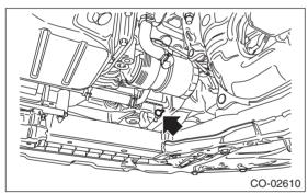
4) Install the drain plug.
