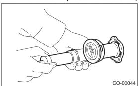
3) Increase pressure until the radiator cap tester gauge needle stops. Radiator cap is functioning properly if it holds the service limit pressure for 5 — 6 seconds. Replace the radiator cap if its valve opens at less than the service limit.
