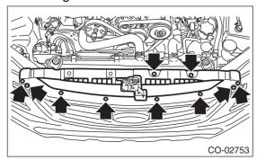
5) Install the air intake duct. <Ref. to IN(H6DO)-8, INSTALLATION, Air Intake Duct.>
