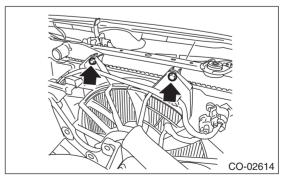
14) Remove the radiator fan shroud.
