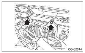
2) Install radiator inlet hoses LH and RH to the radiator.
