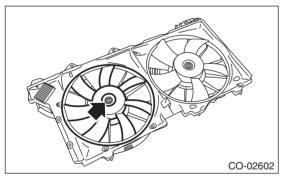
3) Remove the radiator sub fan motor.
