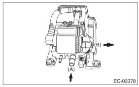
3) Connect the battery positive terminal to the terminal No. 5 and the battery negative terminal to the terminal No. 1. Check that air does not come out from (B) when air is blown into (A).
