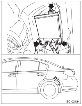
7) Disconnect the vent tube (A), canister drain tube (B) and charge tube (C) from the canister.
