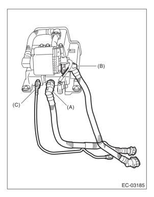
8) Disconnect the connector (A) from the leak check valve assembly, and remove the connector assembly from the canister clip.
