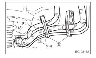
6) Disconnect the connector (A) from the canister and remove the canister from the vehicle.
