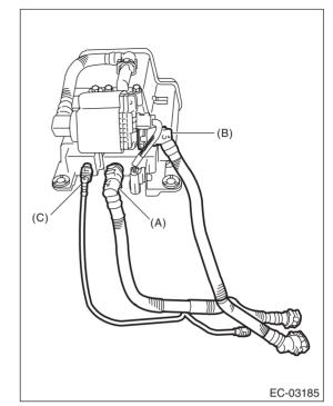
3) Install the canister to the vehicle, and connect the connector (A) to the canister.
