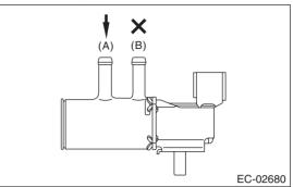
4) Connect the battery positive terminal to the terminal No. 1 and the battery negative terminal to the terminal No. 2. Check that air is discharged from (B), when supplying air to (A).
