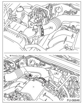
5) Remove the air intake boot assembly, and move it to the left side wheel apron.
