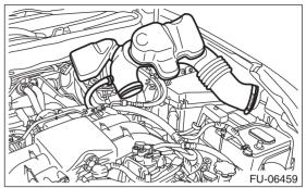
6) Disconnect the connector and hoses of purge control solenoid valve, and then remove the purge control solenoid valve.
