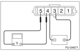
2) Check that the voltage changes when air is blown to the mass air flow sensor unit from arrow direction.
