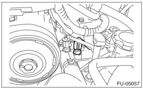
4) Remove the oil temperature sensor.
