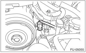
5) Remove the engine coolant temperature sensor.
