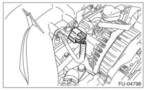
4) Remove the manifold pressure sensor and the filter and hose from intake manifold.
