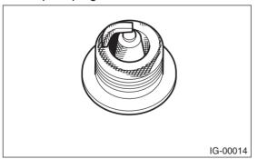
3) Using a nylon brush, etc., clean and remove the carbon or oxide deposits from the spark plug. If deposits are too stubborn, replace the spark plugs. After cleaning the spark plugs, check the spark plug gap "L" using a gap gauge. If it is not within the standard, replace the spark plug.
