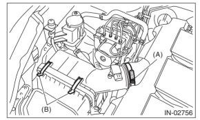
6) Pull the air cleaner case (rear) backward of the vehicle, and remove the air cleaner element.
