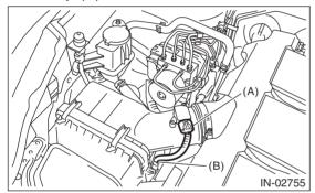
4) Loosen the clamp (A) which connects the air cleaner case (rear) and air intake boot assembly.5) Remove the clip (B) securing the upper side of air cleaner case.
