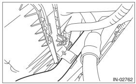
3) Disconnect the connector (A) from the mass air flow and intake air temperature sensor, and remove the clip (B).
