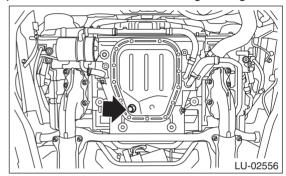
5) Tighten the engine oil drain plug after draining engine oil.
