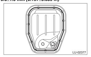
2) Tighten the oil pan lower installing bolts in the numerical order as shown in the figure.
