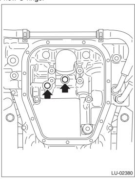
2) Apply liquid gasket to the mating surfaces of strainer.
