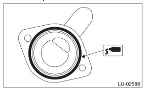
3) Install the strainer to the oil pump.
