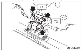
4) Remove the lifting device and wire ropes.
