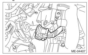
13) Connect the connector to the throttle body.
