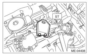
10) Install the throttle body to intake manifold.
