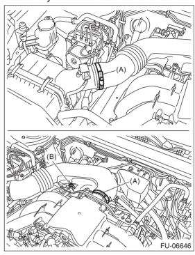
5) Remove the air intake boot assembly, and move it to the left side wheel apron.
