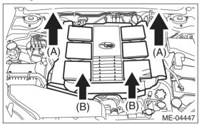
3) Loosen the clamp (A) which connects the air intake boot assembly.
