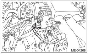
15) Remove the engine harness connector from the engine hanger bracket.
