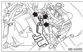
17) Remove the throttle body from the intake manifold.
