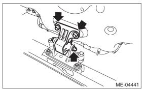
21) Remove the front mounting bracket from the cradle.
