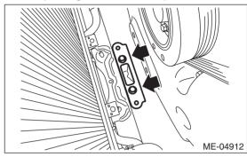
2) Install front mounting bracket to the cradle.
