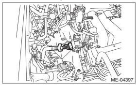
14) Disconnect the connector from the throttle body.
