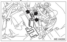
12) Install the engine harness connector to the engine hanger bracket.
