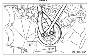
3) Remove the crank pulley.
