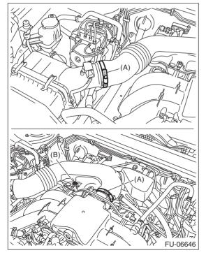
10) Remove the air intake boot assembly, and move it to the left side wheel apron.
