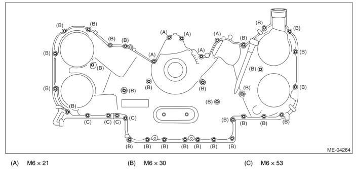
4) Tighten the chain cover installing bolts in the numerical order as shown in the figure.
