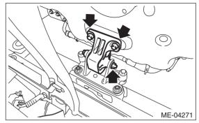
26) Remove the front mounting bracket from the cradle.
