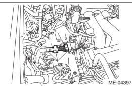
20) Install the V-belts. <Ref. to ME(H6DO)-51, IN-STALLATION, V-belt.> 21) Install the air intake boot assembly.
