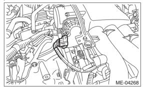
14) Remove the engine harness connector from the engine hanger bracket.
