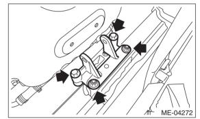
27) Remove the oil cooler pipe from the chain cover.
