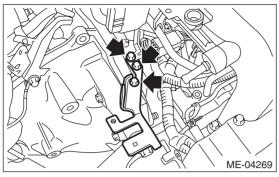
16) Remove the throttle body from the intake manifold.
