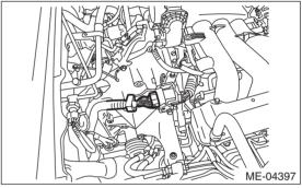
13) Disconnect the connector from the throttle body.
