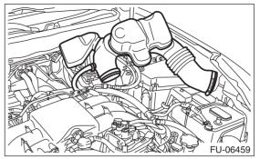
11) Remove the air intake duct. <Ref. to IN(H6DO)-8, REMOVAL, Air Intake Duct.>
