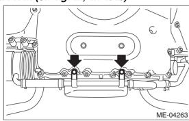
6) Install front mounting bracket to the cradle.
