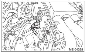
19) Connect the engine harness connector.
