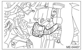
18) Connect the connector to the throttle body.
