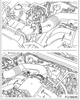
22) Install the air intake duct. <Ref. to IN(H6DO)-8, INSTALLATION, Air Intake Duct.>
