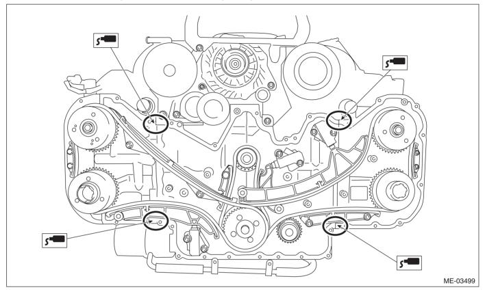
2) Apply liquid gasket to the mating surface of the chain cover.
