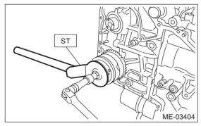
6) Remove the cam sprocket.
