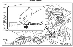
(2) Connect the fuel pressure gauge with ST1 and ST2.
